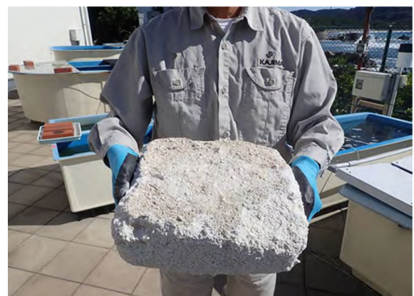
FIGURE 13 Consolidated block of carbonate sand and gravel in an outdoor aquarium. Dimensions: 30 cm x 30 cm x 12 cm; weight: 13.5 kg.
