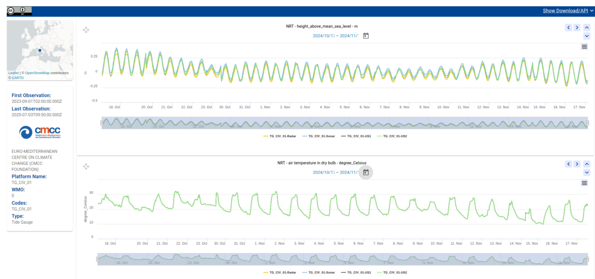
FIGURE 20 One-month time series of sea level data displayed on EMODnet Physics and recorded at Civitavecchia, Italy.
