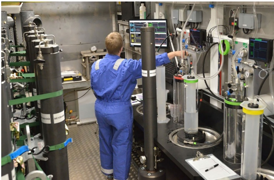
FIGURE 9 Depressurization laboratory for high-throughput quantitative core (Schultheiss et al., 2017).
