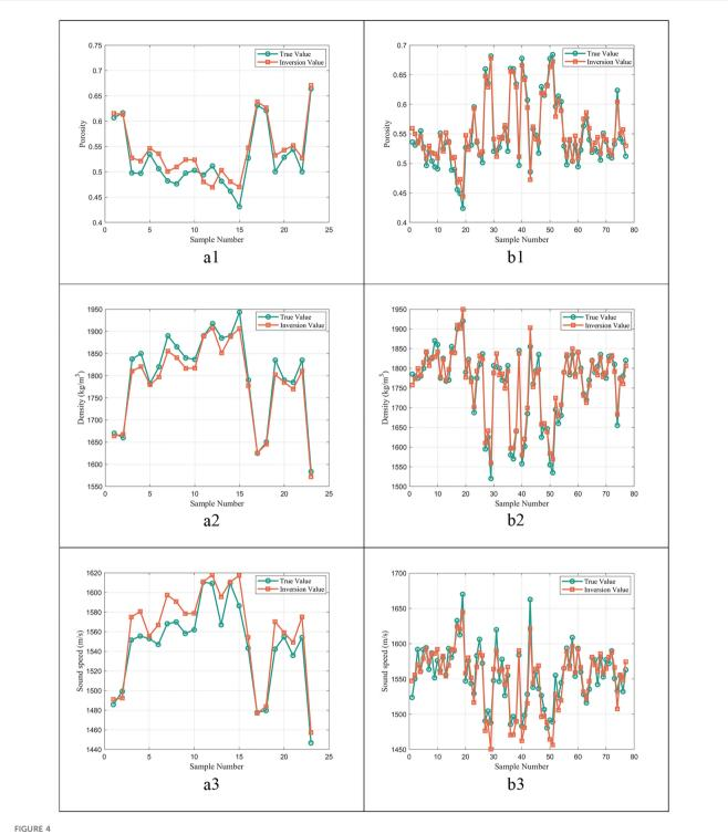
Inversion results under different frequency conditions: (a1) Porosity inversion results at 8 kHz; (a2) Density inversion results at 8 kHz; (a3) Velocity inversion results at 8 kHz; (b1) Porosity inversion results at 100 kHz; (b2) Density inversion results at 100 kHz; (b3) Velocity inversion results at 100 kHz.
