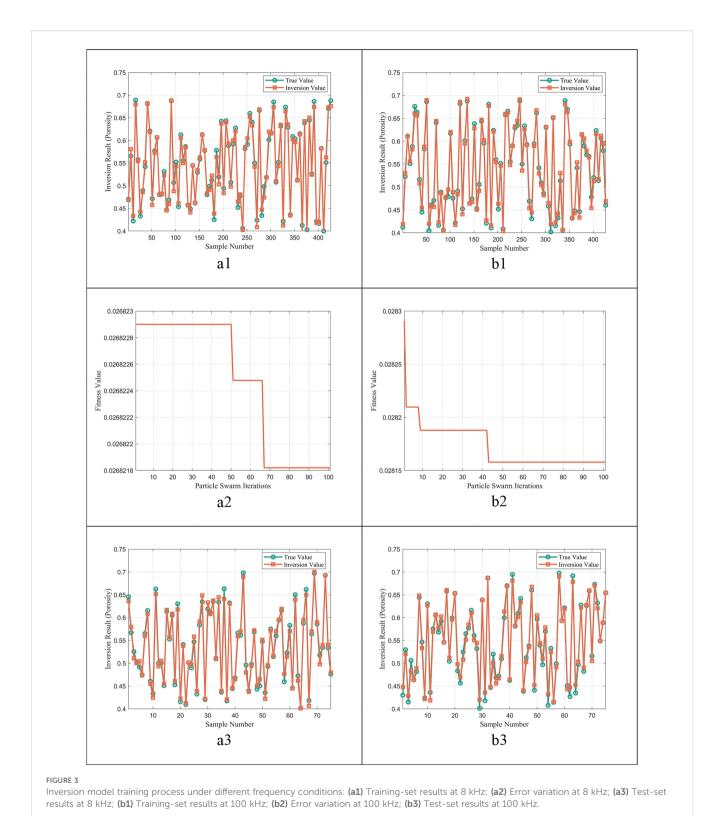
The training results (shown in Figures 3a1, 3b1) display plots of sample number (horizontal axis) versus the predicted porosity obtained from the inverse model (vertical axis). The true porosity values, obtained via forward modeling, are plotted as the actual data, while the predicted values are derived from the trained neural
