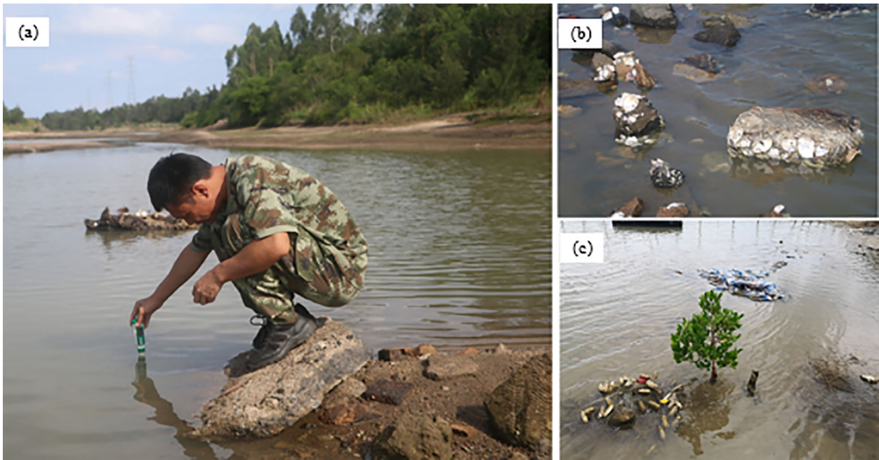
FIGURE 5 Field validation of wetlands in estuarine waters: (a) field salinity measurements; (b, c) marine organisms (oysters, mangrove seedlings) judging salinity and lightness demarcation points.
