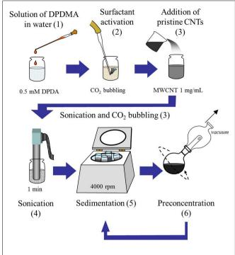
SCHEME 1 | Flow chart depicting the protocol for the preparation of MWCNTs suspensions. Note that the numbers indicate each representative step as detailed in the "Materials and Methods" section above.
