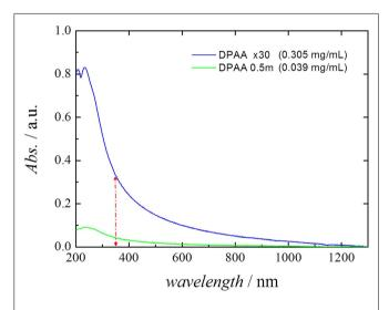
FIGURE 3 | UV-Vis-NIR spectra of the different stable CNT dispersions employed in the present study, after 1:35 dilution in water. The difference between the absorbance at 1300 nm (baseline) and 350 nm was used as the indicative parameter for determining the CNT concentration.
