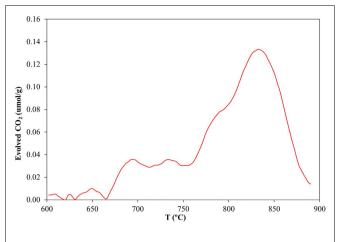
FIGURE 6 |  $CO_2$  desorption rate profile as a function of temperature during the combustion of a CNT-loaded silica capillary tube described in this study in synthetic air.
