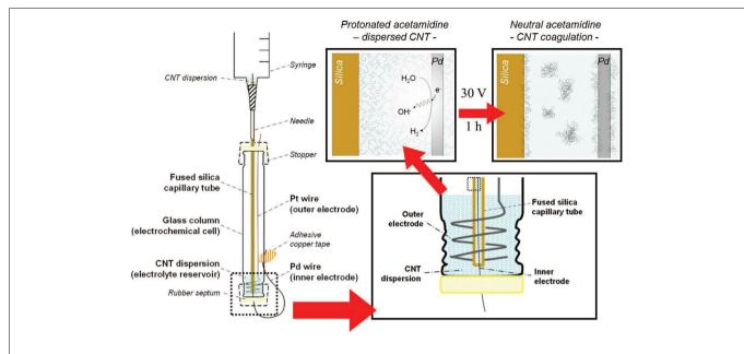
FIGURE 2 | Illustration of the experimental set-up for the electrochemically assisted deposition of MWCNTs inside the capillary tubes used in this study. Insets show a close-up view (lower right) of the lower section of the cell and the suggested deposition process (top right).
