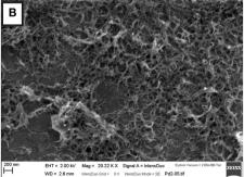
FIGURE 5 | Electron micrographs showing (A) general top-view of the surface of the capillary after undergoing EPD (Scale bar 10 μm) and (B) close-up view of the CNT coating showing a large number of CNT bundles covering the capillary surface (Scale bar 200 nm).
