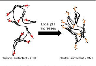
FIGURE 7 | Schematic view of a MWCNT protected by DPDMA and its behavior depending on the pH of the solvent.
