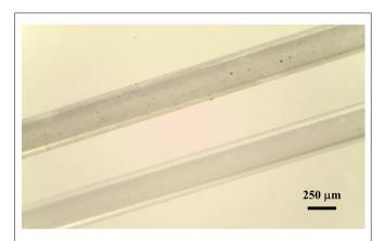
FIGURE 4 | Optical microscopy image of the pristine silica capillary before (bottom) and after (top) undergoing EPD using a MWCNT suspension as described in the Materials and Methods section. Note that the orange polyimide coating covering the outer surface of the capillary has been burned off.
