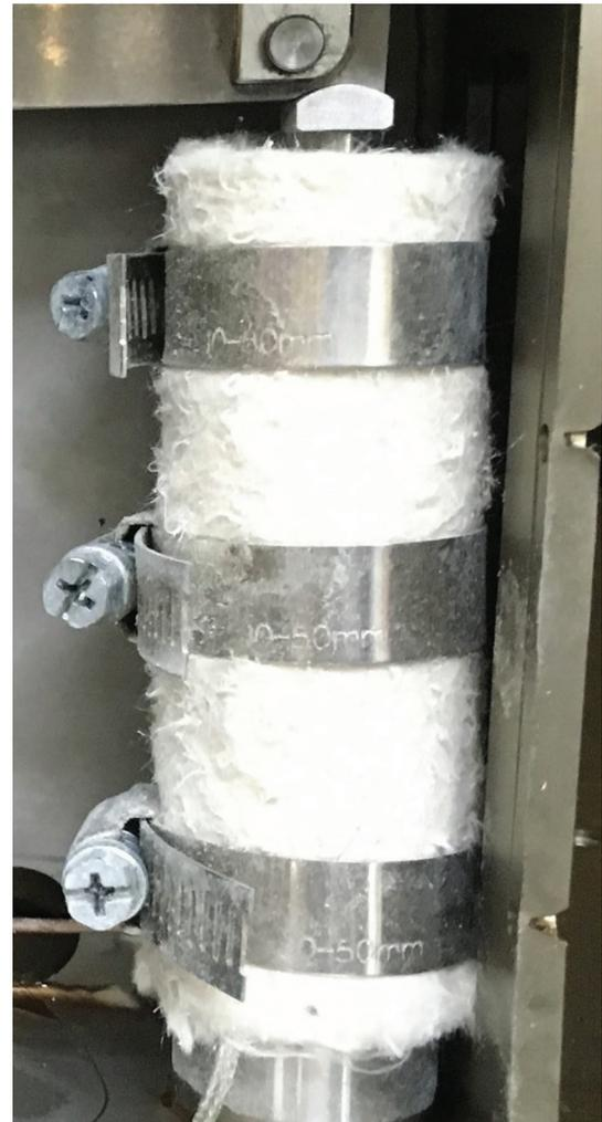
**FIGURE 7 | Photograph of the piezostack actuator with the heat insulation.**
