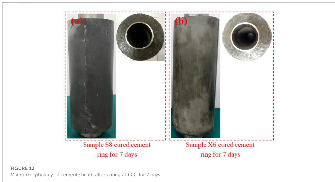
FIGURE 13 Macro morphology of cement sheath after curing at 60C for 7 days.
