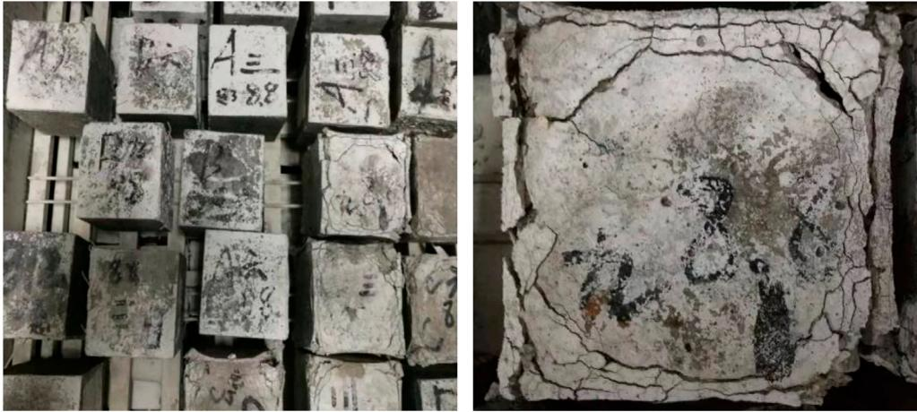
**FIGURE 2** | Picture of concrete specimen damaged by sulfate wetting–drying cycles.
