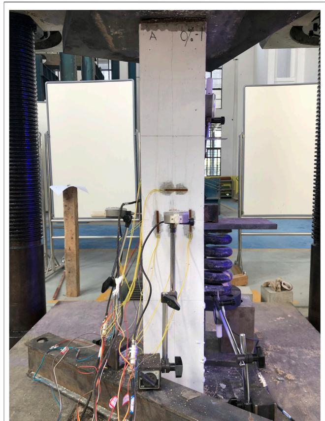
**FIGURE 4** | Loading set-up of the axial compression test.
