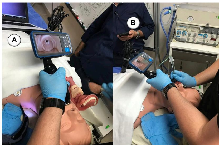
**FIGURE 14 |** Test in the upper airway simulator with the *VidLa-SZ* video-laryngoscope: **(A)** vision of the entrance of the glottis and **(B)** insertion of the endotracheal tube.
