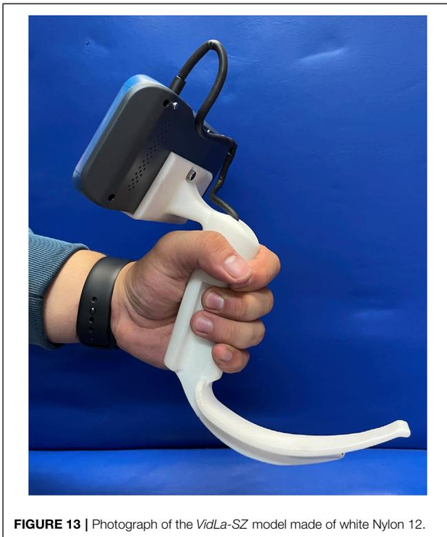
**FIGURE 13** | Photograph of the *VidLa-SZ* model made of white Nylon 12.
