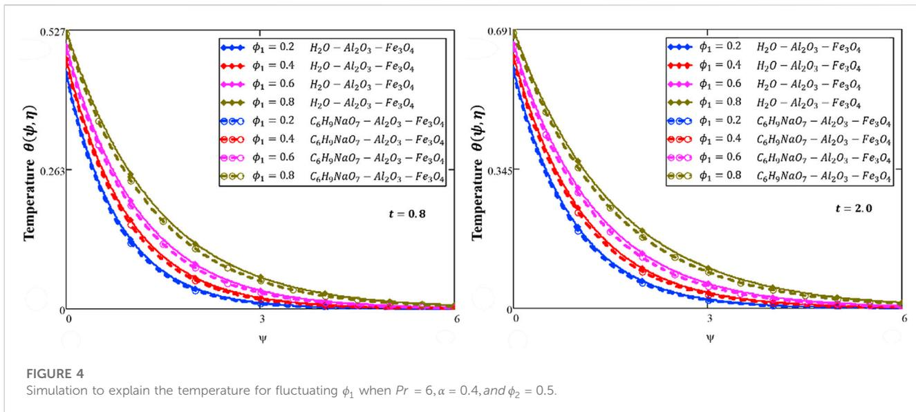
FIGURE 4 Simulation to explain the temperature for fluctuating  $\phi_1$  when  $Pr = 6, \alpha = 0.4,$  and  $\phi_2 = 0.5$ .
