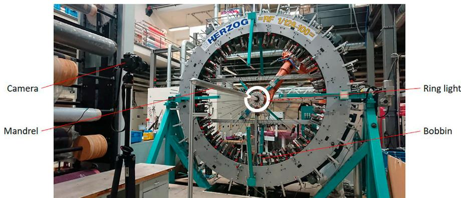
**FIGURE 3** Experimental setup of the RF 1/128–100 braiding machine from HERZOG GmbH equipped with a ring light behind the braid formation zone, a cylindrical mandrel that is overbraided with carbon yarns and a camera that monitors the illuminated braid formation zone.
