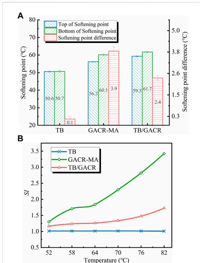
FIGURE 9 Softening point difference (A) and SI (B) of modified asphalts.
