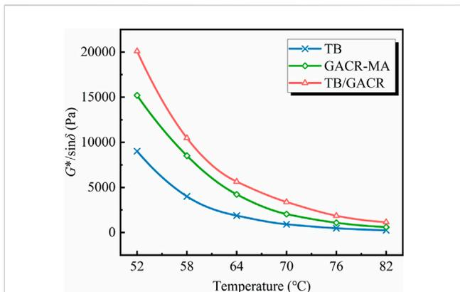
FIGURE 8 The  $G^*/\sin\delta$  of modified asphalt.
