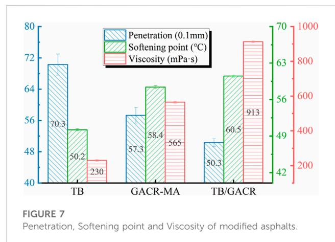
**FIGURE 7** Penetration, Softening point and Viscosity of modified asphalts.
