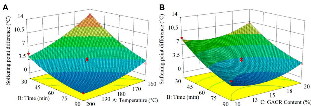
**FIGURE 5** Response surface plot of softening point difference (A) Under the interaction of temperature and time; (B) Under the interaction of time and GACR content.
