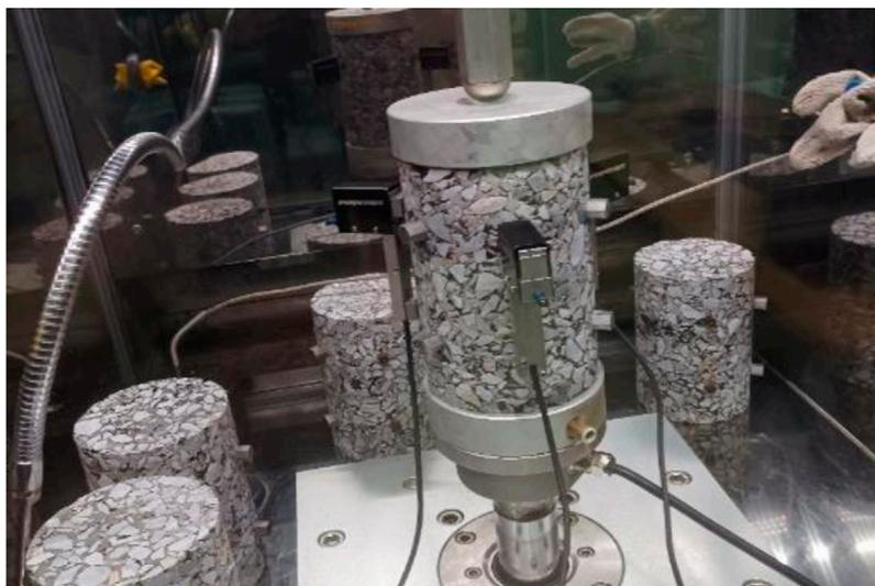
FIGURE 2 Dynamic modulus testing.
