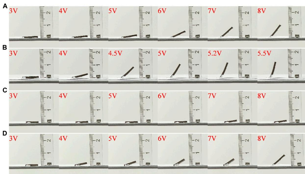
**FIGURE 6** Displacement responses of the soft magnets for different mass ratios and connection methods, (A) AEC, mass ratio = 1, (B) AEC, mass ratio = 2, (C) OEC, mass ratio = 1, (D) OEC, mass ratio = 2.
