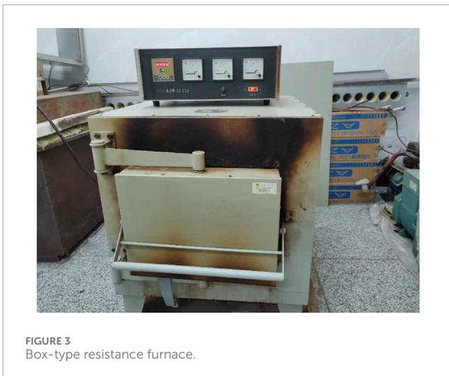
FIGURE 3 Box-type resistance furnace.
