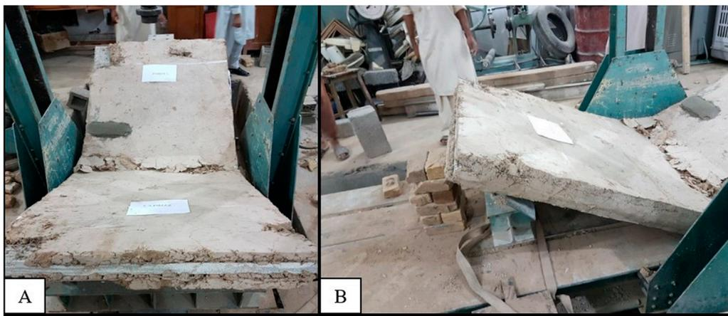
FIGURE 8 Collapsed FP-2 (A) top view (B) side view.
