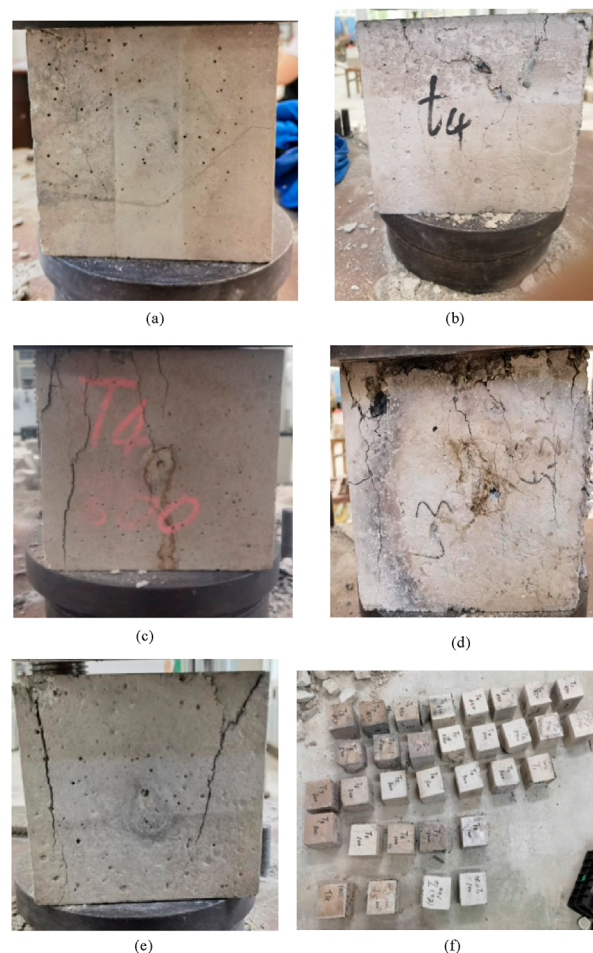
FIGURE 8 Compressive failure morphology of LC30V 4.5 cubes at different temperatures. (a) 25°C, (b) 100°C, (c) 25°C, (d) 100°C, (e) 700°C, and (f) Compressive failure at different temperatures.
