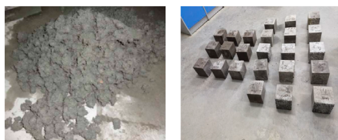
FIGURE 4 The mixture of BFRLC and the surface of the specimen.
