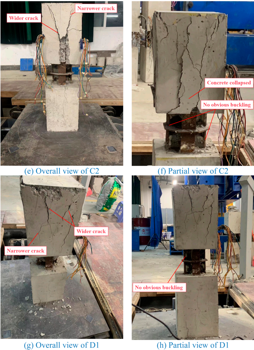
FIGURE 4 (Continued). Test failure mode. (a) Overall view of A1. (b) Partial view of A1. (c) Overall view of B3. (d) Partial view of B3. (e) Overall view of C2. (f) Partial view of C2. (g) Overall view of D1. (h) Partial view of D1.
