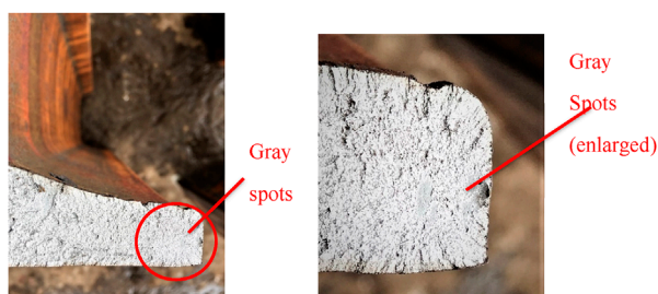
FIGURE 8 Macroscopic morphology of gray spots at the hammer fracture of the flash welding head.
