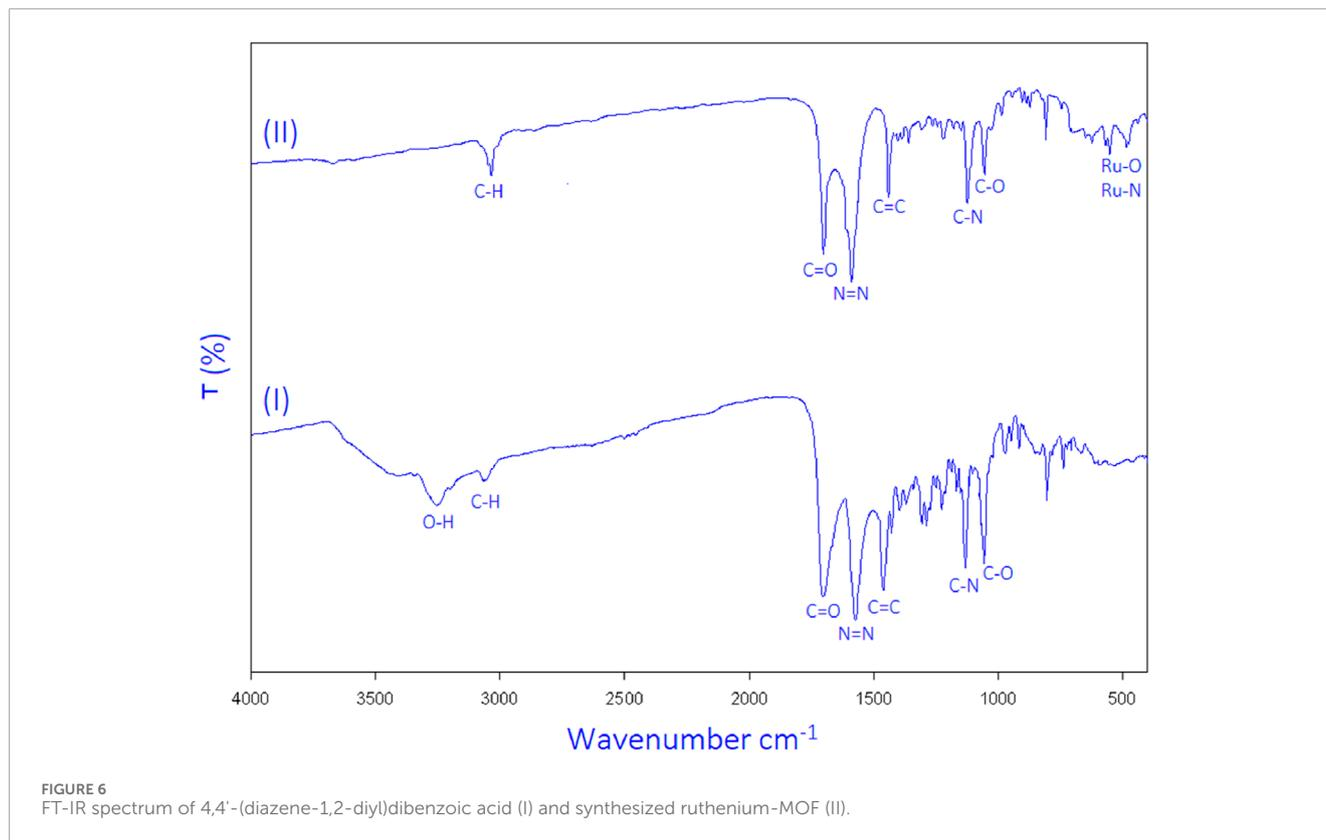
observed in this area, so Ru-N and Ru-O are sites of ruthenium complexation with the 4,4'-(diazene-1,2-diyl)dibenzoic acid, as seen in the FTIR spectrum of the ruthenium-MOF.
