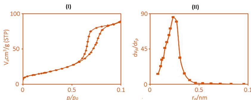
FIGURE 1 Nitrogen adsorption and desorption curve of synthesized ruthenium-MOF [(I): BET, b (II): BJH].
