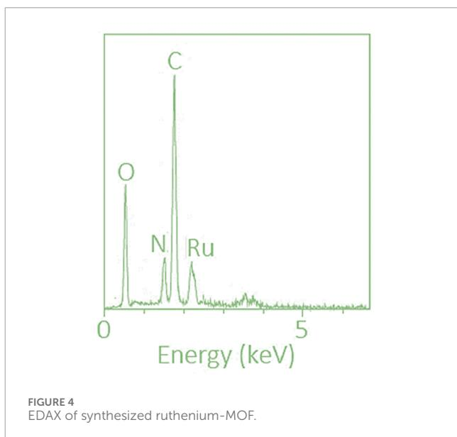
Scanning electron microscopy (SEM) and energy-dispersive X-ray spectroscopy (EDAX): Conducted using a TESCAN VEGA 3 at 15 kV with a working distance of 10 mm in high vacuum mode.
