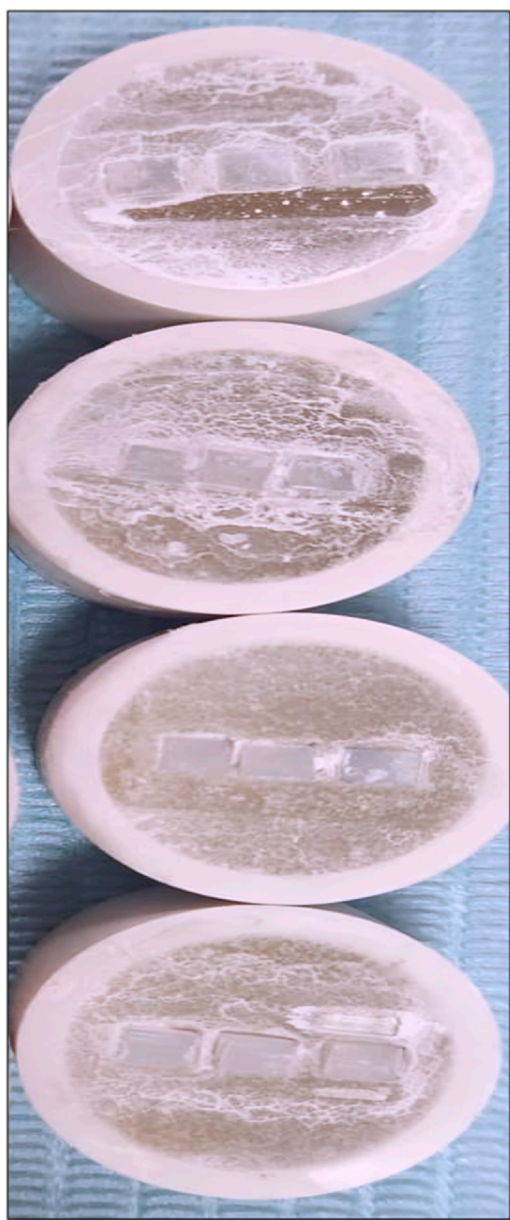
FIGURE 7 Example of composite resin rectangular attachments of the mounted sample post intervention.
