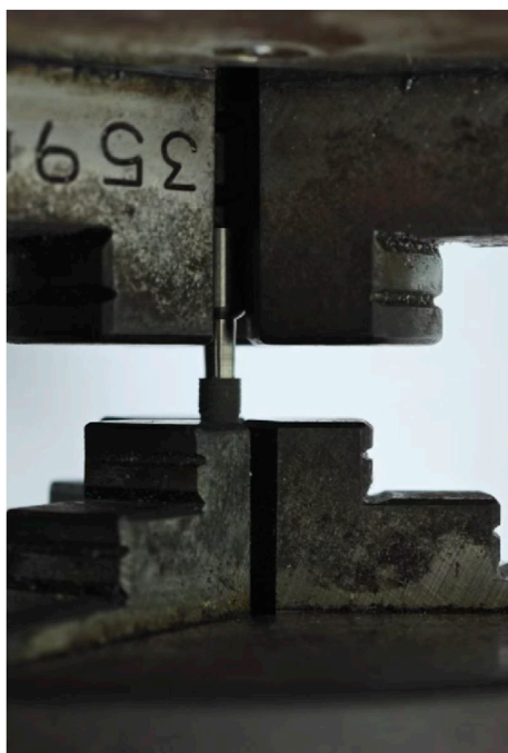
FIGURE 5 Setup for the axial pull-out test.
