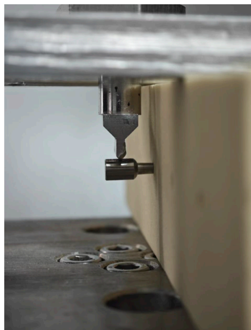
FIGURE 6 Setup for the lateral load test.
