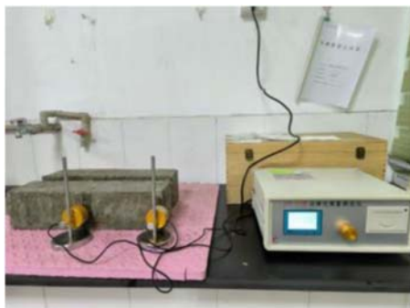
FIGURE 8 Dynamic elastic modulus determination for composite-coated concrete specimens.
