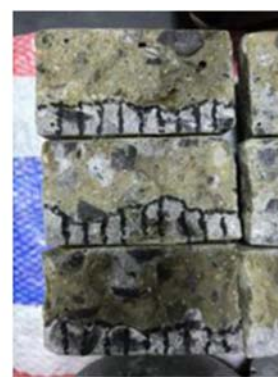
Concrete specimens with silane-cementitious penetration crystallisation composite coating
