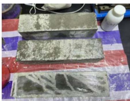
Application of silane impregnation material
