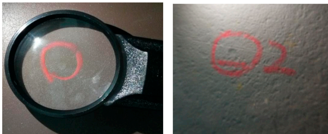
FIGURE 5 Condition of epoxy-60% zinc coating film after impact testing.
