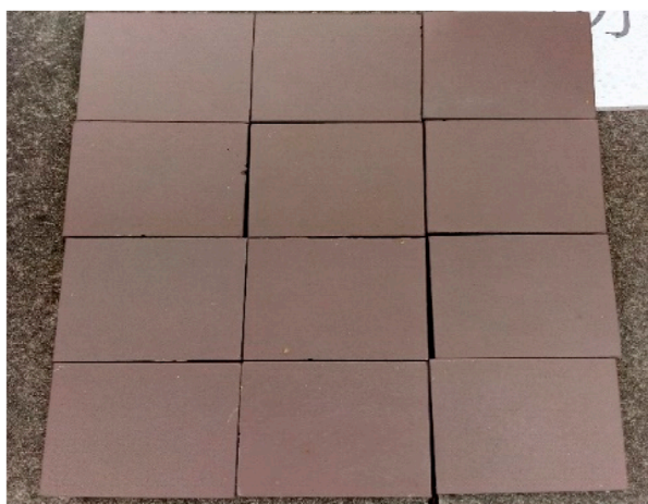
FIGURE 16 Specimen "steel plate + epoxy-60% zinc coating" under natural environmental exposure.
