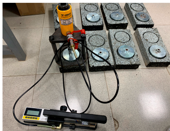
FIGURE 17 Interlayer pull-off test.
