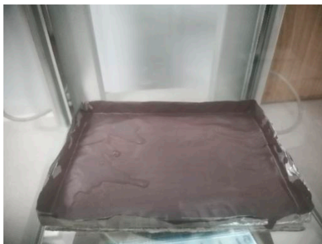
(a) Application of epoxy-60% zinc coating on the carrier plate
