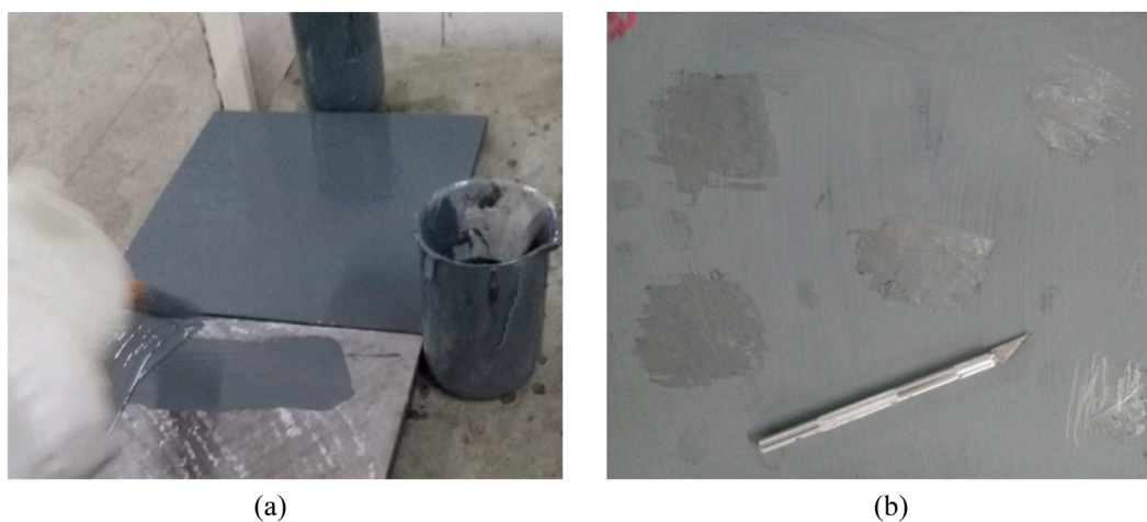
FIGURE 4 Viscosity test process of epoxy-60% zinc coatings: (a) apply epoxy-60% zinc coatings on the steel plate, (b) measure the drying time of the epoxy-60% zinc coatings.
