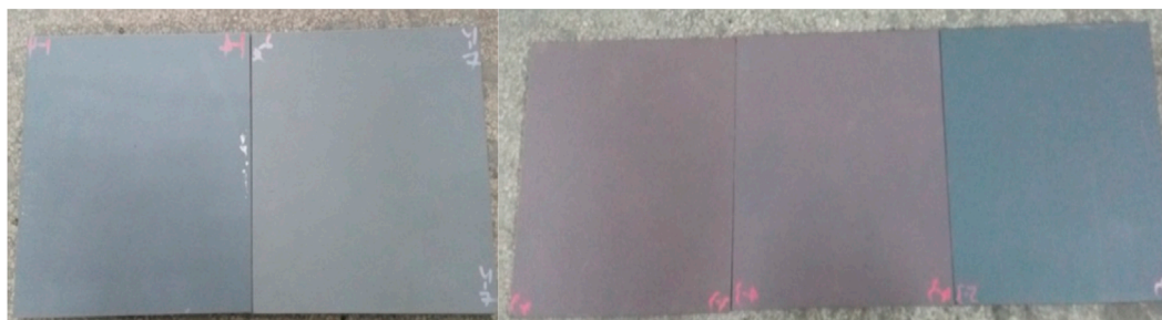
FIGURE 8 Condition of the coating film of the five types of epoxy-60% zinc coatings after heat resistance testing.
