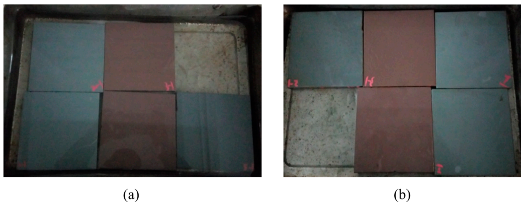
FIGURE 7 "Steel plate + epoxy-60% zinc coating" saltwater immersion test: (a) during the immersion process, (b) after completion of the immersion.
