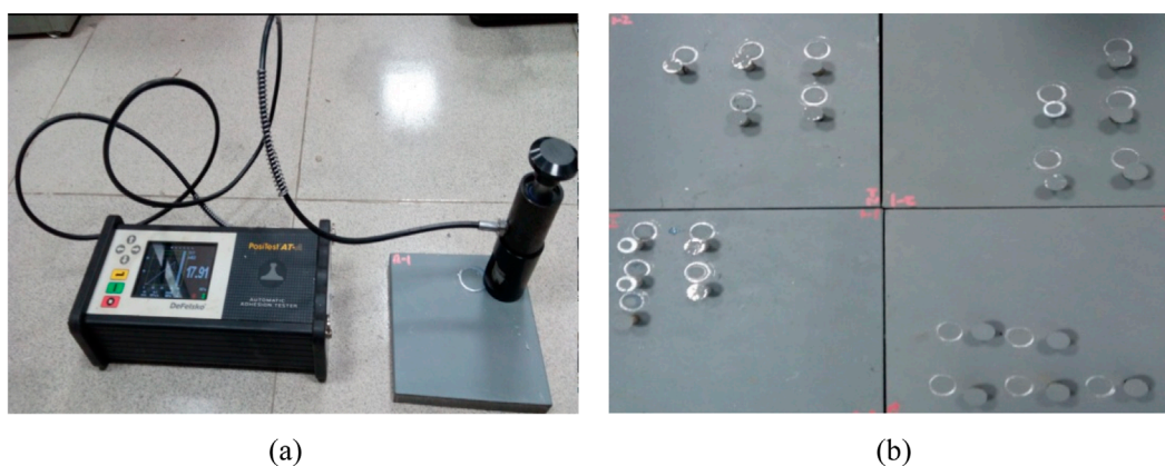
FIGURE 6 Adhesion test procedure of epoxy-60% zinc coatings: (a) adhesion testing equipment, (b) interface failure condition after pull-off test.
