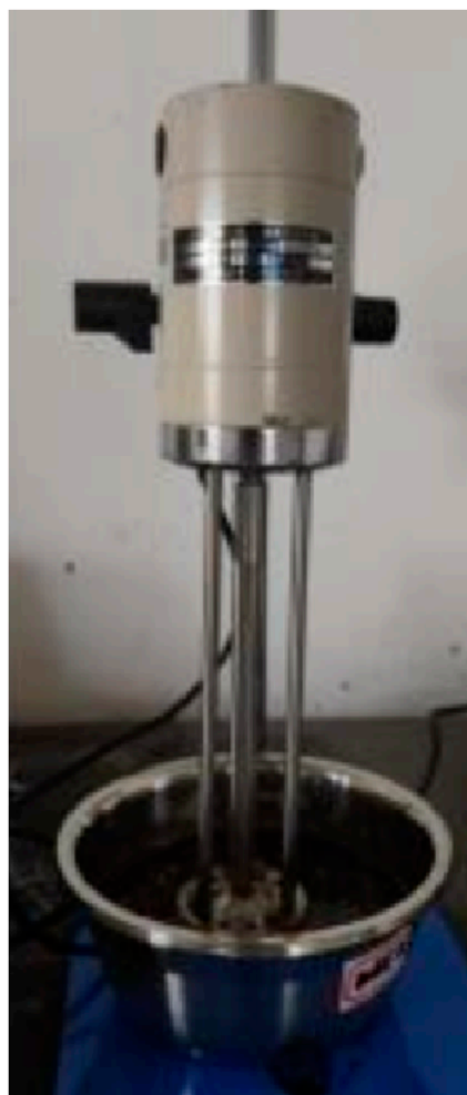
FIGURE 1 Shearing process of modified asphalt.
