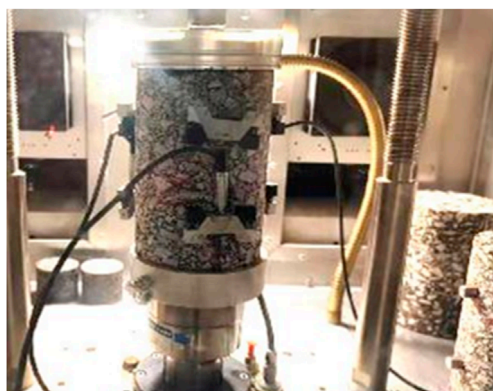
FIGURE 23 Dynamic modulus test loading process.
