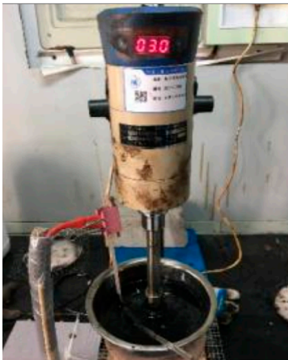
FIGURE 2 Preparation setup for regenerated asphalt.
