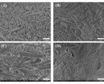
Li<sub>2</sub>Si<sub>2</sub>O<sub>5</sub> glass-ceramics with different compositions
