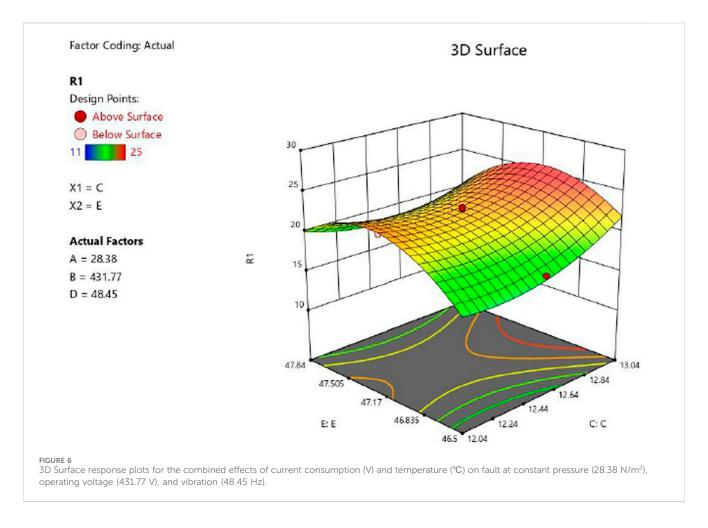
Where A, B, C, D, and E represent the coded values of Pressure, Operating Voltage, Current, Machine Vibration, and Temperature. In the mathematical model, a positive (+) sign signifies a synergistic effect, while a negative (–) sign indicates antagonistic effects on generated faults.
