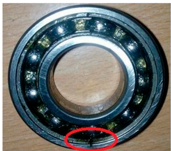
FIGURE 3 Solo defect on outer race.
