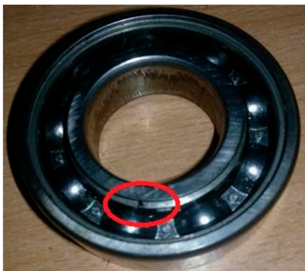
FIGURE 2 Solo defect on inner race.
