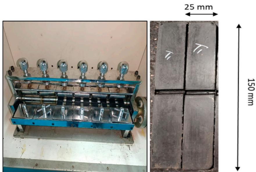
FIGURE 13 Ross flex test machine with test specimen.
