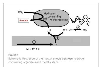
geological environments that can reduce the corrosion rate of container materials. There is a type of hydrogen consuming microorganism in the natural environment that uses hydrogen oxidation as the energy for its life activities. This provides a new approach for us to study reducing the HE sensitivity of nuclear waste container materials (Figure 2).
