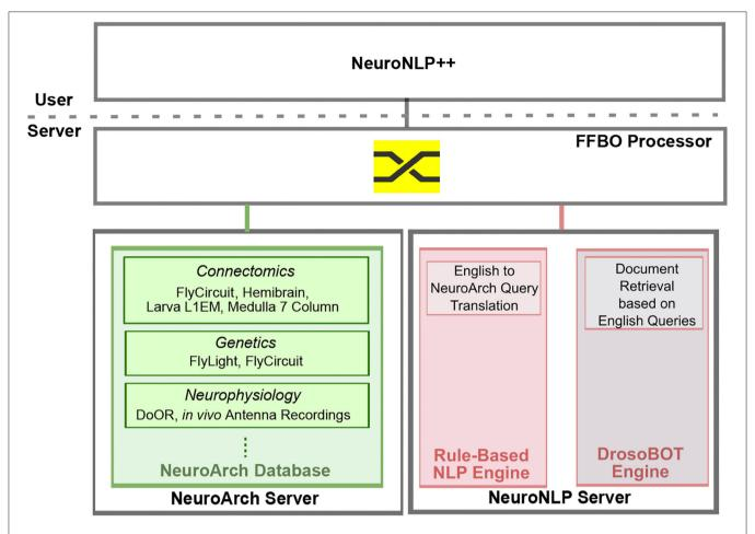
FIGURE 12 | Software architecture of the NeuroNLP++ web application. The frontend application communicates with three backend servers: a NeuroArch Server that hosts a NeuroArch Database of fruit fly brain datasets, a NeuroNLP Server that runs the rule-based NLP Engine, and, an additional NeuroNLP Server that runs the DrosoBOT Engine.
