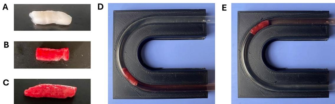
FIGURE 3 Dynamically formed (A) 0%, (B) 25%, and (C) 50% hematocrit EAs used in SR MT flow loop testing. Examples of 50% hematocrit EAs lodged in (D) U-1 and (E) U-2 locations of the U-shape model, respectively.
