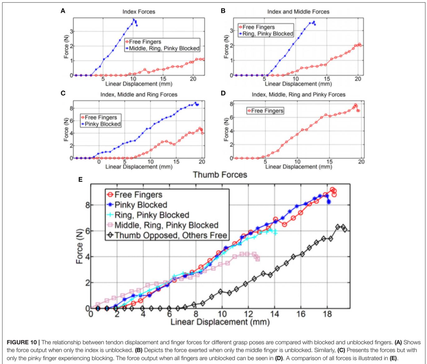
outputs are allowed to move continuously. When one or more outputs is blocked, the series elastic differential can only provide displacements up to 43 mm.
