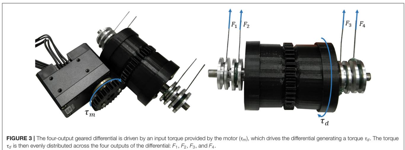
**FIGURE 3 |** The four-output geared differential is driven by an input torque provided by the motor ( $\tau_m$ ), which drives the differential generating a torque  $\tau_d$ . The torque  $\tau_d$  is then evenly distributed across the four outputs of the differential:  $F_1$ ,  $F_2$ ,  $F_3$ , and  $F_4$ .
