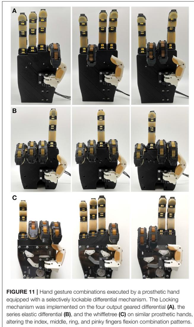
**FIGURE 11 |** Hand gesture combinations executed by a prosthetic hand equipped with a selectively lockable differential mechanism. The Locking mechanism was implemented on the four output geared differential (A), the series elastic differential (B), and the whiffletree (C) on similar prosthetic hands, altering the index, middle, ring, and pinky fingers flexion combination patterns.
