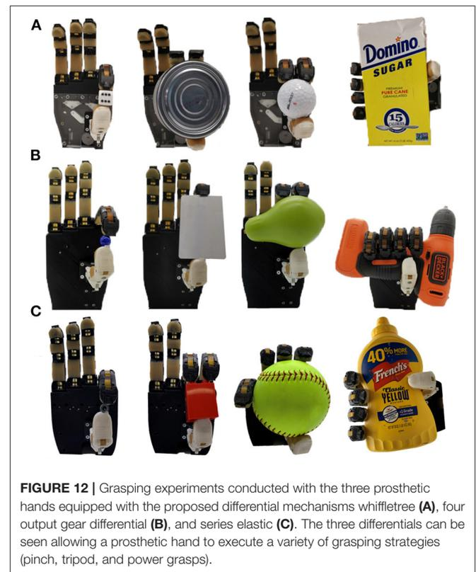
**FIGURE 12 |** Grasping experiments conducted with the three prosthetic hands equipped with the proposed differential mechanisms whiffletree (A), four output gear differential (B), and series elastic (C). The three differentials can be seen allowing a prosthetic hand to execute a variety of grasping strategies (pinch, tripod, and power grasps).
