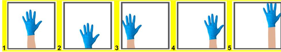
**FIGURE 4 |** Hand Listener: commands issued to the drone via hand gestures. The offset of the hand with respect to the center indicates the planar direction toward which the drone has to move. The five hand position examples in the figure indicate that the drone should move respectively: forward (1), backward (2), rightward (3), leftward (4), and forward-leftward (5).
