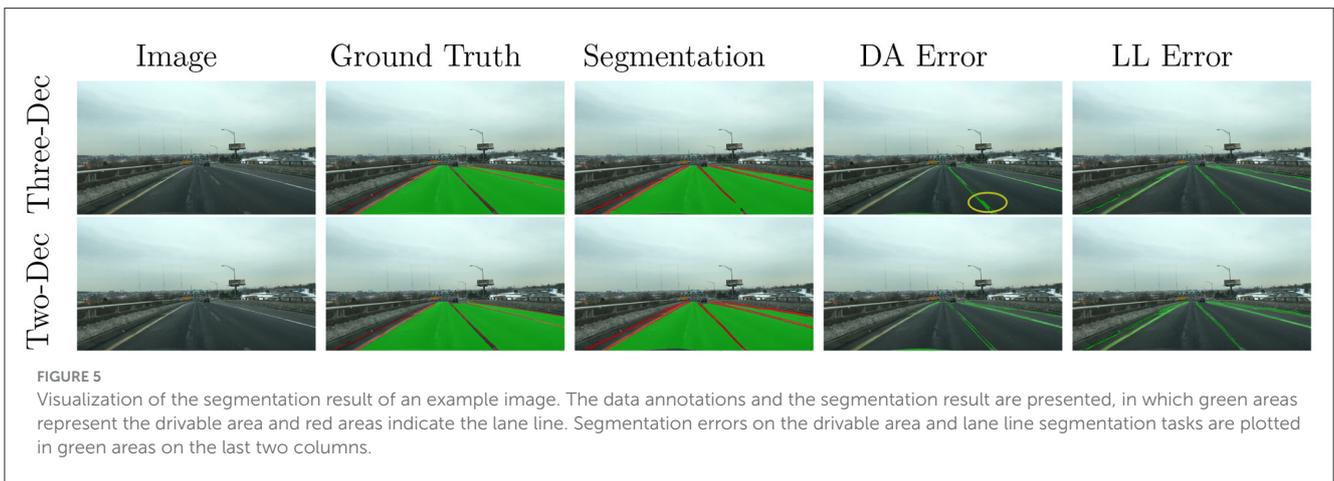
FIGURE 5 Visualization of the segmentation result of an example image. The data annotations and the segmentation result are presented, in which green areas represent the drivable area and red areas indicate the lane line. Segmentation errors on the drivable area and lane line segmentation tasks are plotted in green areas on the last two columns.
