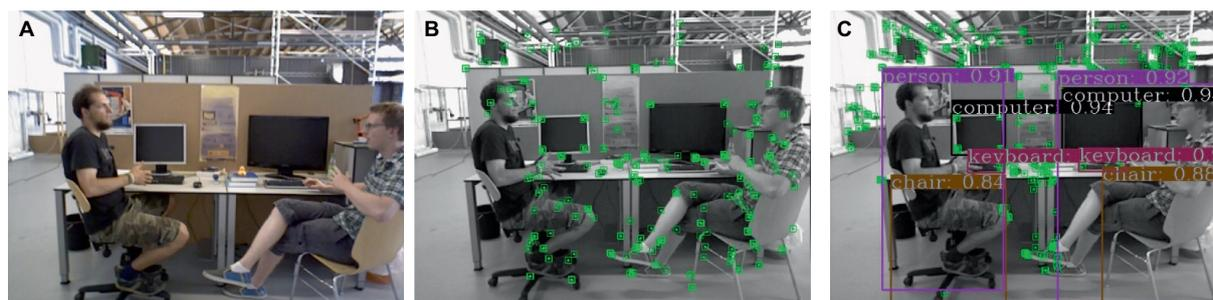
FIGURE 9 The comparison of feature point extraction between the proposed algorithm and the ORB-SLAM3 algorithm.
