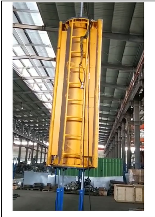
FIGURE 12 Scaled experimental model of the wave compensation system.
