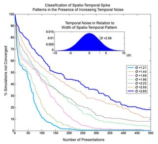
due to temporal noise distribution with standard deviation  $\sigma = 0-1 \Delta t$ . At lower noise levels the convergence profile is approximately the same or faster (red) than the zero noise case. The right panel shows the same for  $\sigma \approx 1-3 \Delta t$ .
