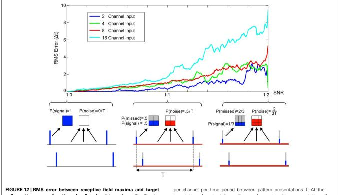
**spike patterns as a function of spike signal to noise ratio.** The three bottom panels show the spike probability distributions at three points along the SNR axis. The signal spikes (blue), missed spikes (gray), and noise spikes (red) are illustrated for the three cases of 1:0, 1:1, and 1:2 signal to noise ratios. The mean spike rate was maintained at 1 spike
