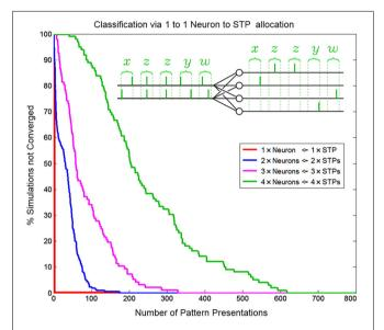
FIGURE 14 | Convergence rate of as a function of neuron/pattern numbers and number of pattern presentations for a 1-to-1 two input neuron to pattern allocating network. As the number of patterns/ neurons increases the system requires longer pattern sequences to correctly allocate exactly one unique pattern to each neuron. The inset shows the five consecutive correct classifications of four patterns by four neurons.
