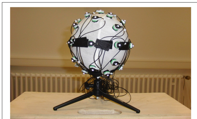
FIGURE 5 | Photo of the fiberglass sphere. Here we can see the fiberglass sphere with the attached electrodes, the covering fabric and the hook straps fixing the electrode cables.
