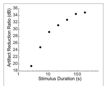
**FIGURE 7** | Dependence of artifact reduction quality on data length. The artifact reduction ratio (ARR, measured between 300 and 6000 Hz) is shown as a function of the data length (varied between 2.7 and 171.8 s in octave steps) used to estimate the Wiener prediction filter for the example of **Figure 5**. The cross-validated ARR increases with increasing data length with a net improvement of ∼2.5 dB per doubling of the data length.
