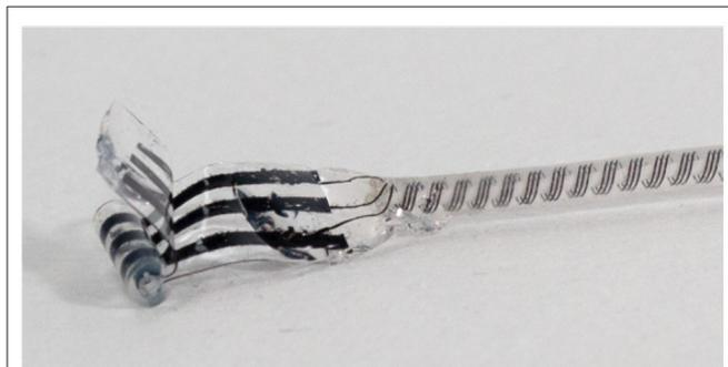
**FIGURE 2** | Elastomer electrode used in *ex-vivo* block and stimulation experiments at Imperial College. The conductive elastomer is black and encased in flexible silicone, with a silastic tube to shape the material into a cylinder for use as a cuff electrode. Material and electrode manufacturing details are provided by Cuttaz et al. (2021). Courtesy of Estelle Cuttaz, Rylie Green research group, Imperial College.
