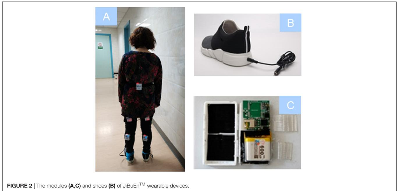
**FIGURE 2 |** The modules (A,C) and shoes (B) of JiBuEn™ wearable devices.
