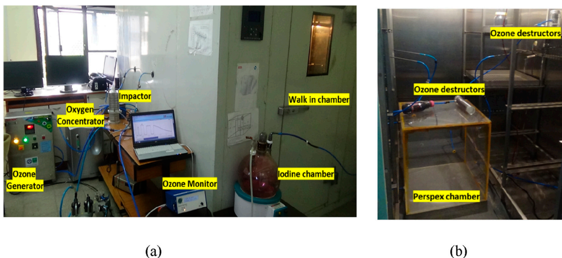
FIGURE 2 Picture of (a) experimental set-up and (b) inside of walk-in chamber.
