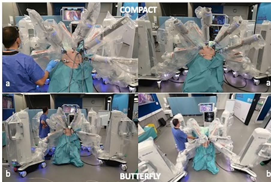
**FIGURE 6 | (A)** The “compact” docking configuration; **(B)** The “butterfly” docking configuration.
