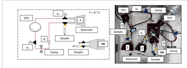
Setup of the *in vitro* hemolysis test circuit (1, 2) with static reference N0: schematic sketch of one test circuit with static reference (left); picture of two test circuits and one static reference (right).
