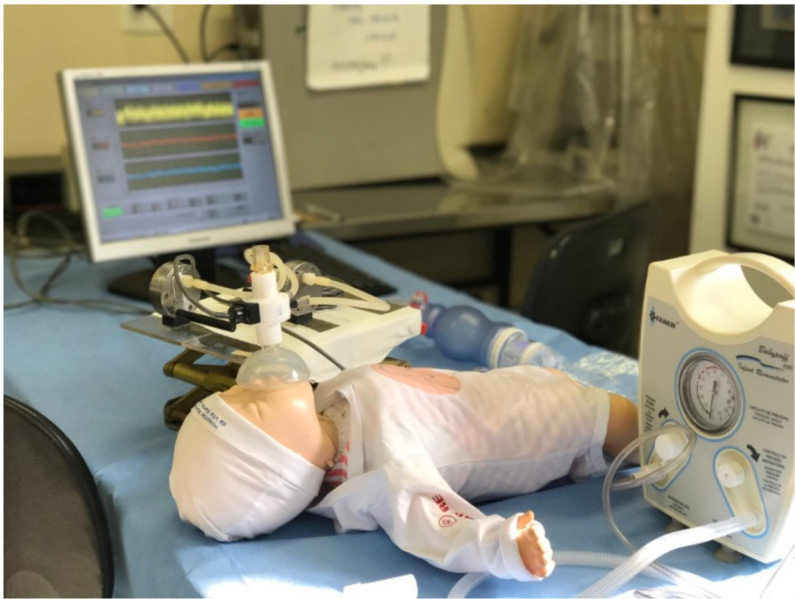
FIGURE 3 Layout of the study as the neonatal manikin's ventilation is assessed by the respiratory function monitor attached to the face mask.
