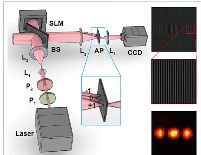
**FIGURE 3** | Experimental setup. P1-P2, polarizers; L1-L4, lens; BS, beam splitter; SLM, spatial light modulator; AP, aperture for filtering; CCD, charge coupled device camera. The blue rectangle highlights the filtering aperture, with the details of extracting +1st-order diffraction component. The right insets exhibit the mask loaded on SLM, enlarged view of the mask, and the experimental pattern recorded by CCD from top to bottom, respectively.
