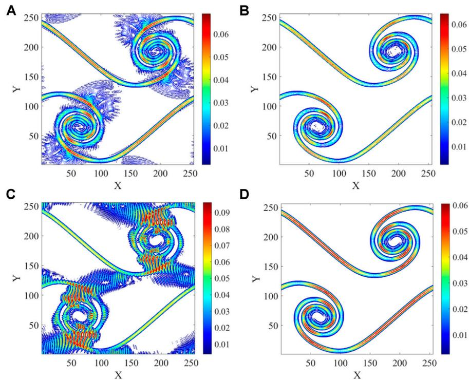
**FIGURE 15** | Filter coefficient contour plot in the double shear layer at  $Pe = 5.12 \times 10^8$  for different schemes: **(A)** FD scheme, **(B)** BGK collision operator, **(C)** PR1st collision operator, **(D)** HR collision operator.
