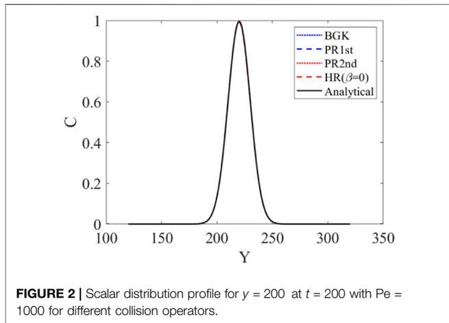
**FIGURE 2** | Scalar distribution profile for  $y = 200$  at  $t = 200$  with  $Pe = 1000$  for different collision operators.
