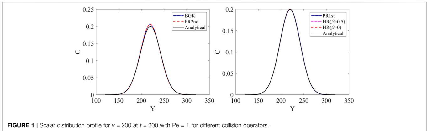
**FIGURE 1** | Scalar distribution profile for  $y = 200$  at  $t = 200$  with  $Pe = 1$  for different collision operators.
