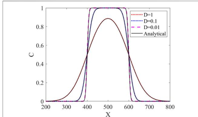
**FIGURE 3** | Scalar distribution profile for  $D = 1, 0.1,$  and  $0.01$  at  $t = 2000$  for the different schemes.
