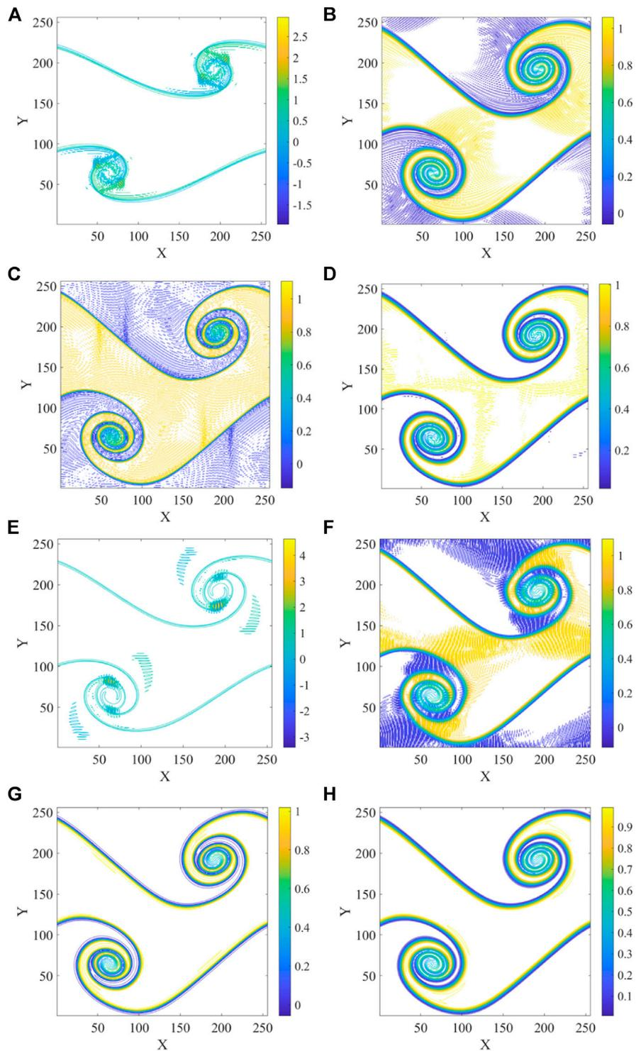
**FIGURE 13** | Unfiltered (left) and filtered (right) results at  $Pe = 5.12 \times 10^8$ . From top to bottom: **(A, B)** FD unfiltered and filtered, **(C, D)** BGK unfiltered and filtered, **(E, F)** PR1st unfiltered and filtered, **(G, H)** HR unfiltered and filtered.
