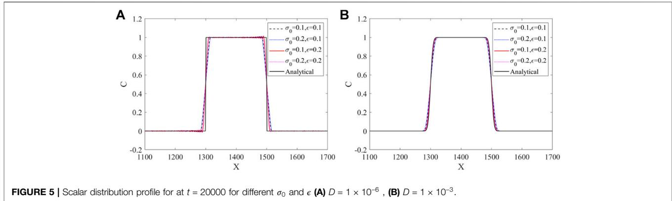
**FIGURE 5** | Scalar distribution profile for at  $t = 20000$  for different  $\sigma_0$  and  $\epsilon$  (A)  $D = 1 \times 10^{-6}$ , (B)  $D = 1 \times 10^{-3}$ .
