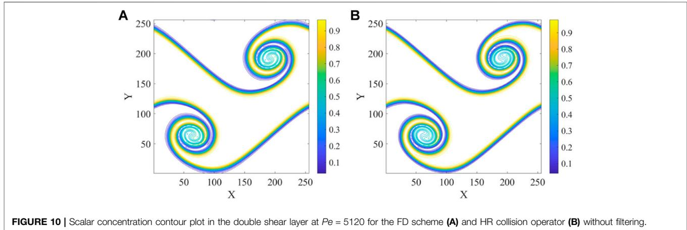
**FIGURE 10** | Scalar concentration contour plot in the double shear layer at  $Pe = 5120$  for the FD scheme (A) and HR collision operator (B) without filtering.
