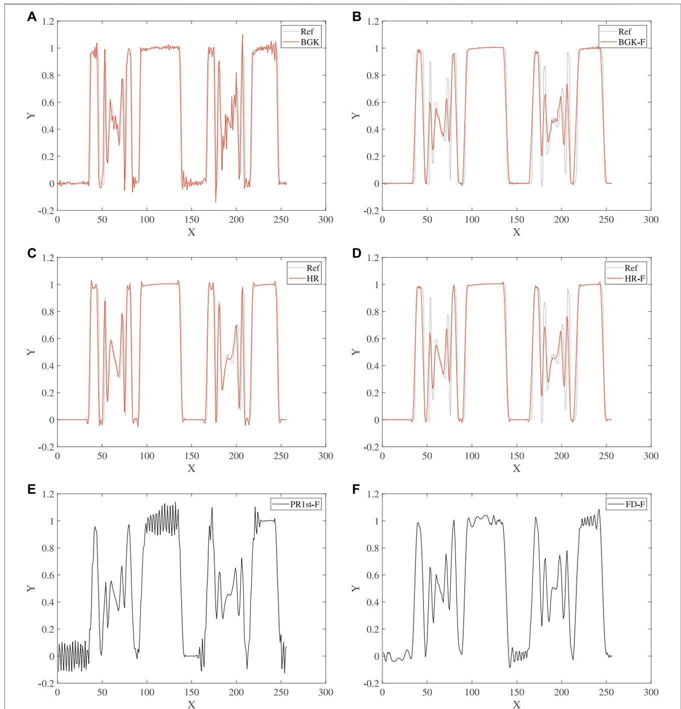
**FIGURE 14** | Scalar distribution profile at  $Pe = 5.12 \times 10^8$  along the counter-diagonal of the domain for different schemes: **(A,B)** BGK unfiltered and filtered, **(C,D)** HR unfiltered and filtered, **(E)** PR1st with filter, **(F)** FD scheme with filter.
